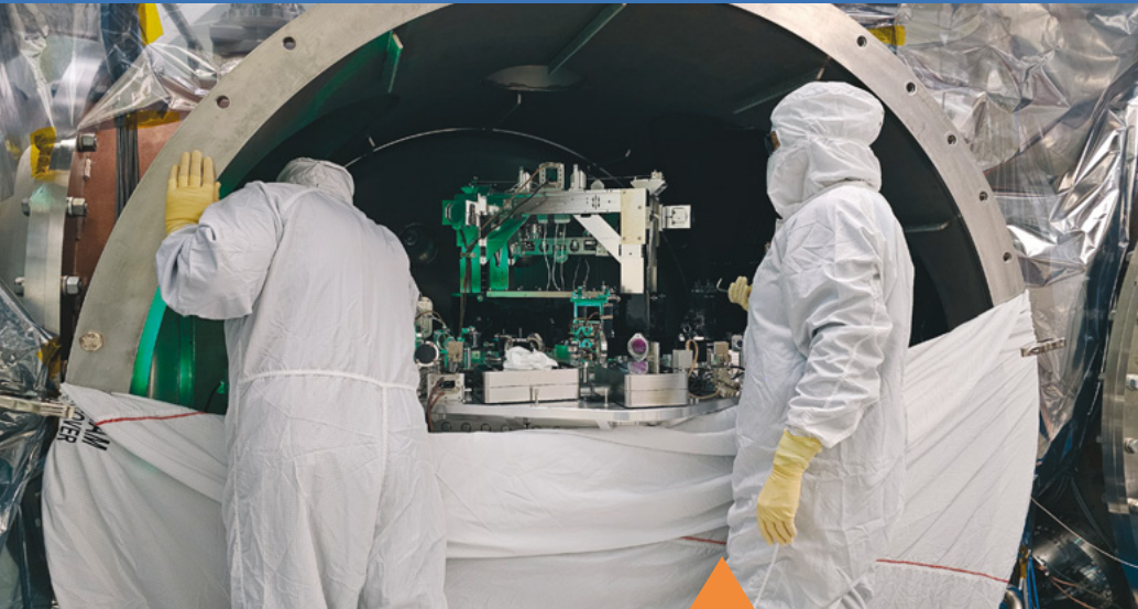
Anamaria Effler and Adam Mullavey inspecting surrounding components for damage caused by the Fast Shutter failure—thankfully, they found no signs of damage!
